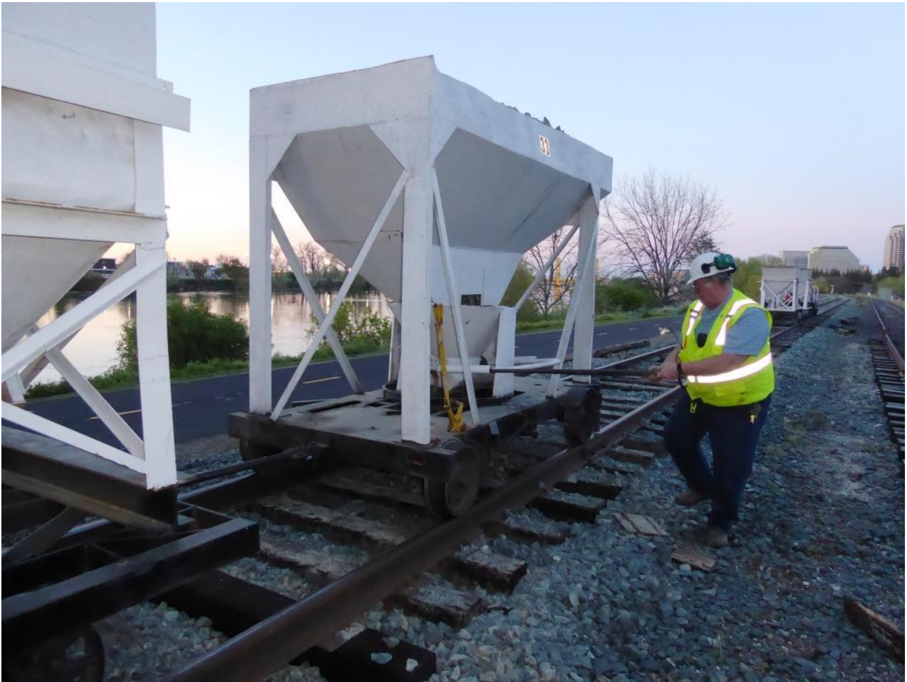
Chris disengages the center-dump car
